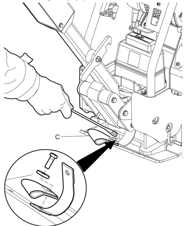
**3. Mount the trolley (D) in the trolley strap (C).**
