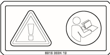
Instruction manual. The operator must read the safety, operation and maintenance instructions before operating the machine.
