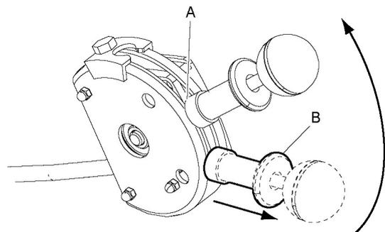
2. Pull out the starter rope until it resists. Release the handle so the starter rope goes back again, and then pull the starter rope until the engine starts.
