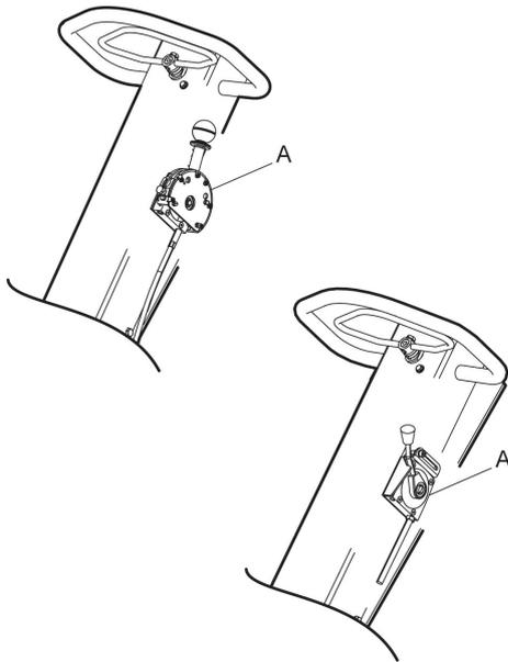
2. Lubricate the controls (A, B) if necessary.
