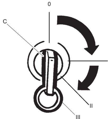
3. Turn the ignition key (C) through position II, to position III.
