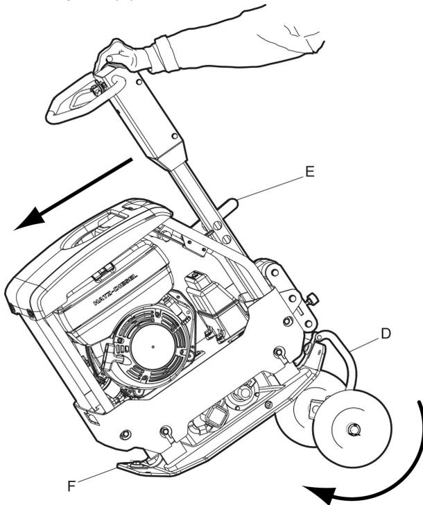
5. Unlock the handle (E) and tilt the machine backwards.
